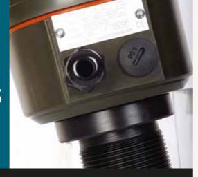
Orion Rotate is used with all powdery and granulated bulk materials of coarse grade, for level monitoring (detection) in all types of containers and silos. It has 8 different adjustable torque settings, which are adjusted using the three position DIP switch.
